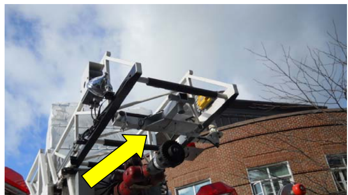
Housing with 5 ultrasonic sensors. The sensors transmit a signal to video screen at the operator's position that shows proximity of ladder to target.
