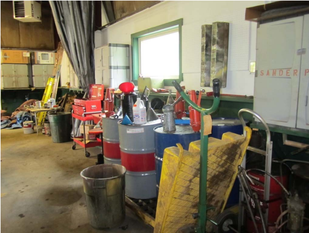
Photograph No. 8: Flammable liquid containers stored in maintenance garage.
