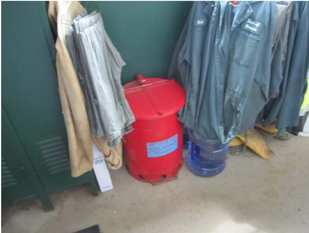
Photograph No. 15: Oily rag container.
